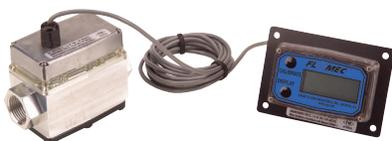
The Factory Mutual (FM) Approved Remote Kit Assembly modifies FLOMEC® Electronic Digital Meters for applications in specialized situations including remote indication and high or low fluid temperature metering applications. This kit provides the versatility of panel mounting of the LCD readout up to 100 ft. (30 m) from the turbine.
